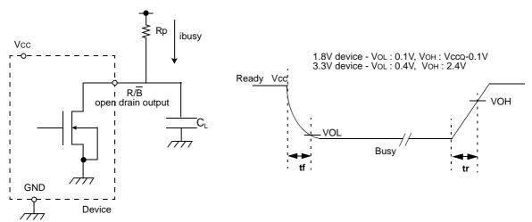
Figure 17. Rp vs tr ,tf & Rp vs ibusy
